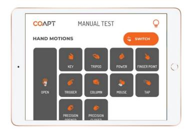
Use Triggers Switches to map requested grips and gestures to the COVVI Hand. Users can access these by providing the previously assigned terminal device Open and Close muscle patterns. All Trigger Switches will be available to select, except 'Co-contraction' as this strategy is not available with any pattern recognition system.
