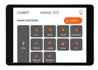
Use Trigger Switches to map requested grips and gestures to the COVVI Hand. All Trigger Switches will be available to select, except 'Co-contraction' as this strategy is not available with any pattern recognition system.
