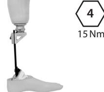
Fit socket to fitting clamp top housing and tighten pyramid screws (15 Nm). Refer to alignment page for initial setup.
