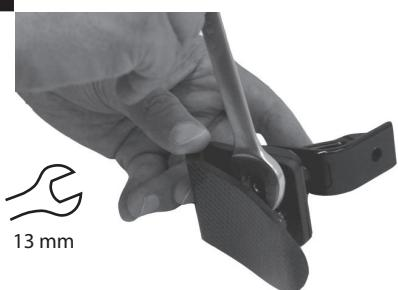
Remove heel spring from carrier.
