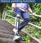
The stance yielding function allows patients to smoothly walk down stairs and slopes step-over-step. In addition, ALLUX 2 allows for individuals to walk with a natural knee flexion movement to help reduce the shock during initial contact with the ground.
