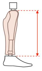
We measure from the level of the foot shell to the top of the knee. The gap between the cover and the foot will be taken into account by us, depending on the type of foot.
