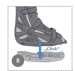
Push both unlocking buttons simultaneously and remove sole. (Fig. 7+8)
