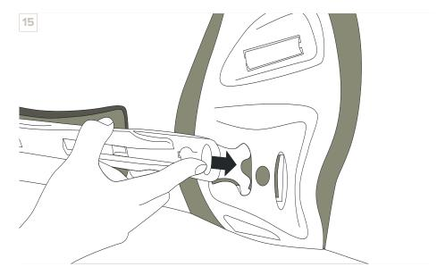
Slide the posterior strut into slot on lumbar belt posterior panel until it snaps into place.
