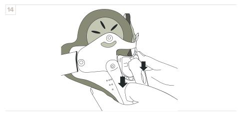
Push down causing strut support to lock into place. Ensure that all three connectors are engaged.
