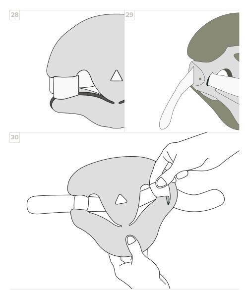
To replace the back pad, begin by attaching the green side of the pad to the hook dots on the back panel. Once the padding is aligned with the plastic, the straps will need to be re-threaded through the padding and plastic slots.
