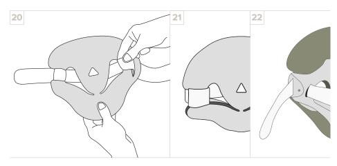
For some of the pads, you must first unthread the straps on each side. To do this, push the straps through the slits in the pad and then through the slots in the outer edge of the plastic. This applies to the collar and lumbar region.
