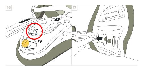
To remove, press the button on the bottom of the posterior connection point on both the collar and the lumbar pad and slide up.
