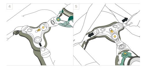
Attach the back panel clips to the sides of the vest. Pull the straps evenly until the back panel is tightened. Adjust the strap padding for comfort.
